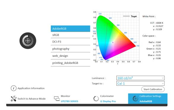
**NOTE:** Calibration settings can be further customized by adjusting "Luminance" and selecting which user profile, i.e. Cal 1/2/3, the calibration result will be saved to.
